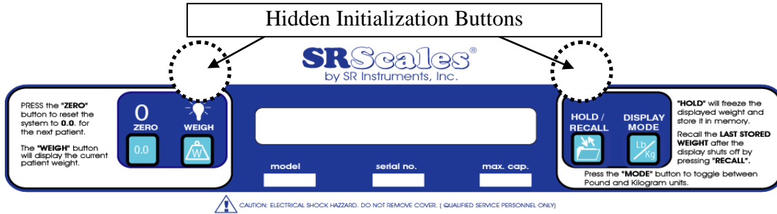
Figure 13: Location of Hidden Initialization Buttons
